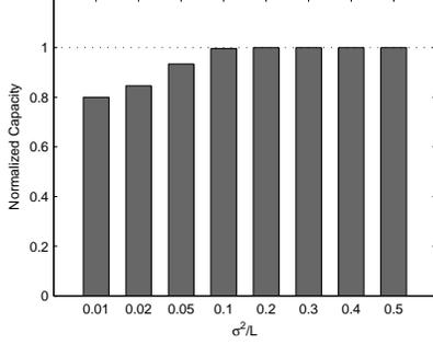
Fig. 10. The gap between system capacity obtained by the proposed scheme and the optimal capacity obtained by brute force searching when  $\sigma^2/L$  varies.
