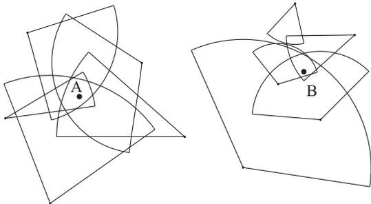
Figure 2. Point A is more likely to be full view covered than point B. When point B faces up, there is no camera closely catching its frontal image.
