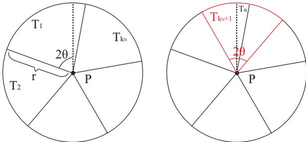
Figure 3. For an arbitrary point  $P$ , the geometric necessary condition of full view coverage is that  $T_1, T_2, \dots, T_{k_{N+1}}$  all have at least one sensor covering  $P$ .
