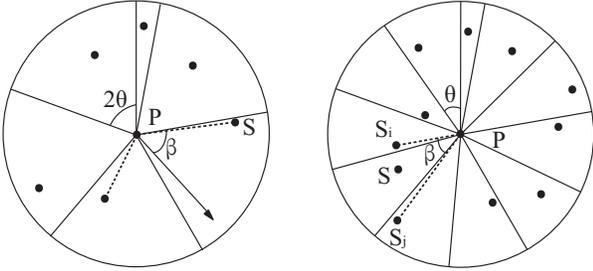
Figure 6. The gap between necessary and sufficient condition – meeting necessary condition does not guarantee full view coverage (left), while in sufficient condition there may be redundancy (right).
