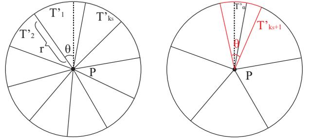
Figure 5. For an arbitrary point  $P$ , the sufficient geometric condition of full view coverage is that  $T'_1, T'_2, \dots, T'_{k_S+1}$  all have at least one sensor covering  $P$ .
