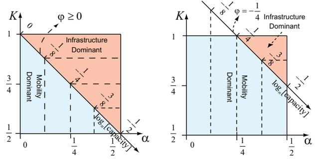
Figure 3: Graphical representation of capacity result in uniformly dense network. We plot per-node capacity as a function of  $f(n) = n^\alpha$  and  $k = \Theta(n^K)$ , with  $\mu^c = \Theta(n^\varphi)$  as parameter. Left plot shows the bottleneck at accessing phase and right plot shows the case that infrastructure network itself is the limitation.
