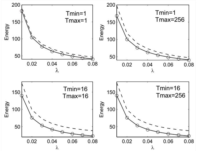
Fig. 4. Energy consumption in terms of  $\lambda$  ( $\lambda_g = \lambda_c = \lambda/2$ ). Solid line: analysis (differentiating frame directions); dashed line: analysis (without differentiating frame directions); symbol: simulation.
