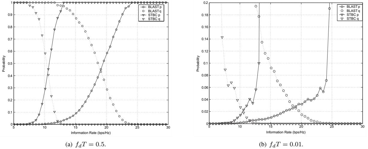
Fig. 2. Gilbert model parameters for  $2 \times 2$  BLAST and STBC for different Doppler values.  $E_s/N_o = 20$  dB.
