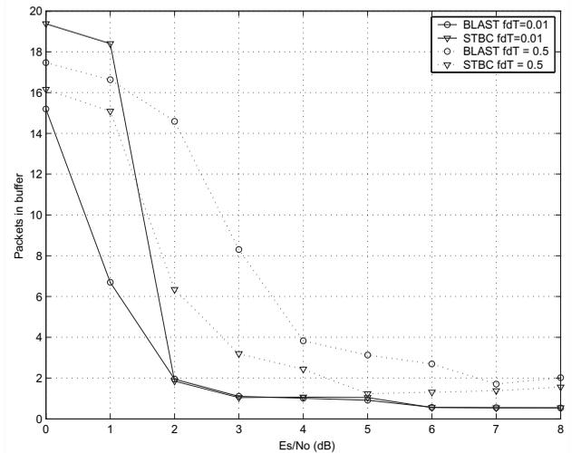
Fig. 8. Average buffer occupancy for  $4 \times 4$  BLAST and STBC operating at the optimal rate for TCP for different Doppler values. Buffer is 30 packets.
