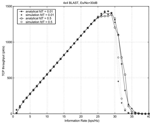
Fig. 3. Comparison of TCP throughput for analytical and simulation results.
