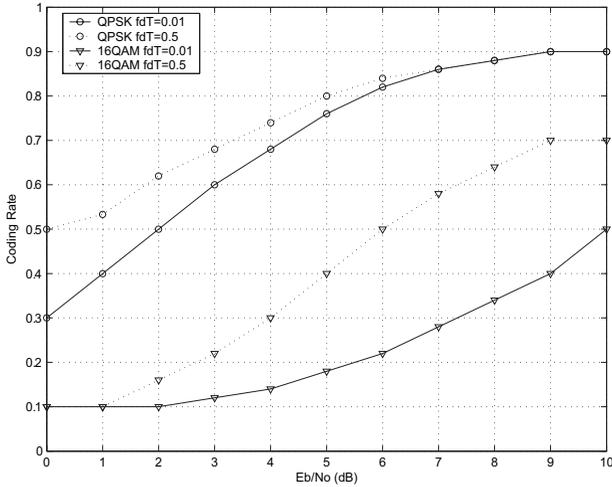
Fig. 6. Optimal coding rate for TCP over  $2 \times 2$  BLAST employing QPSK and 16QAM.
