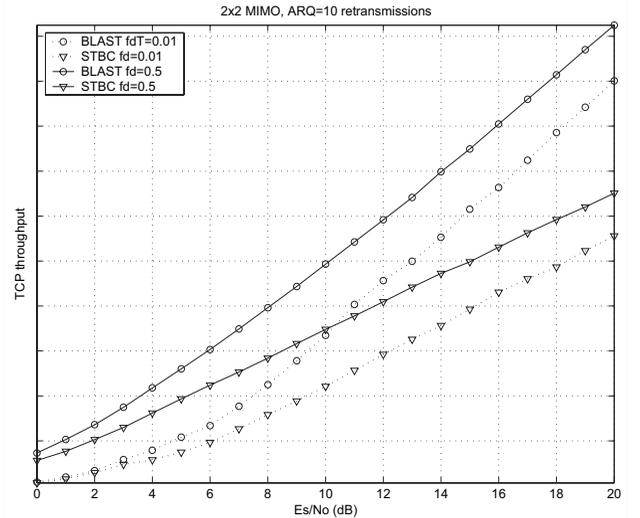
Fig. 5. Comparison of maximum TCP throughput for BLAST and STBC for different Doppler values.
