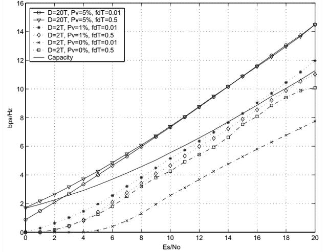
Fig. 9. Rate that maximizes the video throughput for  $2 \times 2$  BLAST under different delay and error constraints.
