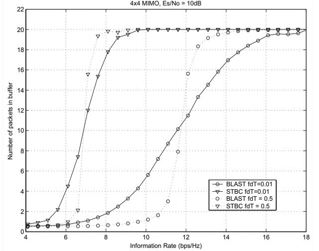
Fig. 7. Comparison of buffer occupancy for  $4 \times 4$  BLAST and STBC for different Doppler values. Buffer is 20 packets and  $E_s/N_o = 10$  dB.
