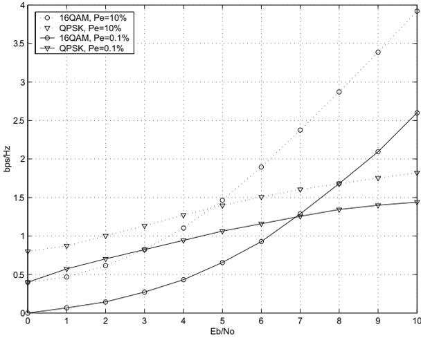
Fig. 10. Video throughput over a  $2 \times 2$  BLAST employing QPSK and 16QAM modulations for different frame error targets. Buffer is 20 packets.
